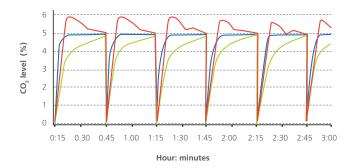
Precisely-tuned sensor and software result in fast recovery of CO<sub>2</sub> without overshoot. This ensures uniform CO<sub>2</sub> levels even with frequent incubator door opening.
