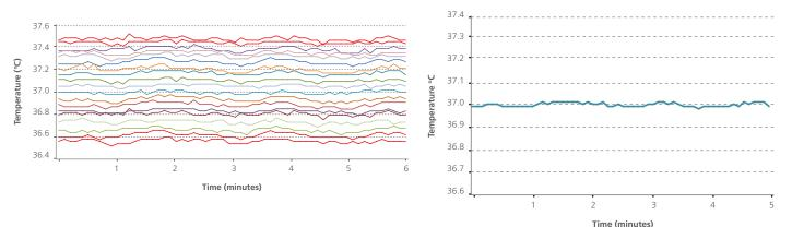
Different lines represent different sensor positions inside the chamber. Esco CelCulture® has uniformity variance of less than  $\pm$  0.5°C which means all the samples are evenly heated.\*
