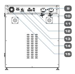
11. Alarm contact 12. Analog output 13.RS485 14. Power supply inlet 15. Cooling fan
